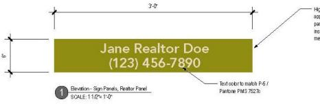
High resolution digitally printed graphic applied to both sides of .09" thick metal panel. Panel attached to mounting tabs on inside of frame with tamper resistant mechanical fasteners.
